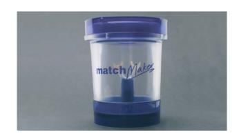
After the investment has set (30 minutes) rotate the base of the former and remove. Gently press the investment from the Matchmaker PRESS pressing ring. Smooth the underside of the ring with a plaster knife. Place in a pre-heated burn-out furnace at 900°C – see investment directions for use.
