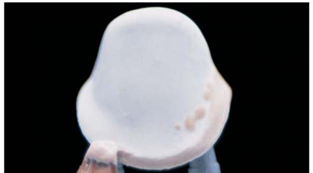
After firing the surface should appear textured with a slight sheen.
