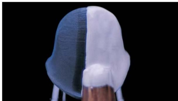
After firing, the surface should have a slight sheen.
