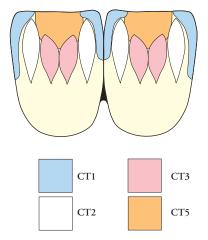
Lay down the Matchmaker ALX Colour Translucent powders using a lateral segmental build up technique. Commonly used Matchmaker ALX Colour Translucent powders are CT1 Blue, CT2 White, CT4 Yellow and CT5 Orange.
